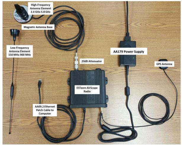
Figure 3: AirScope Connection Diagram
