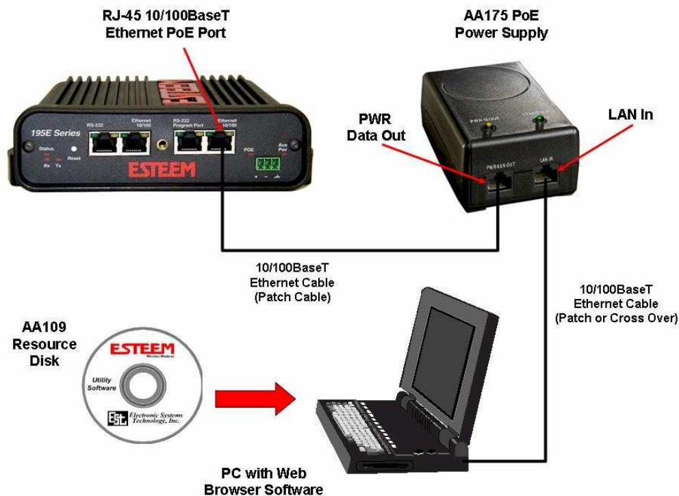
Figure 4: Hardware Configuration Diagram
