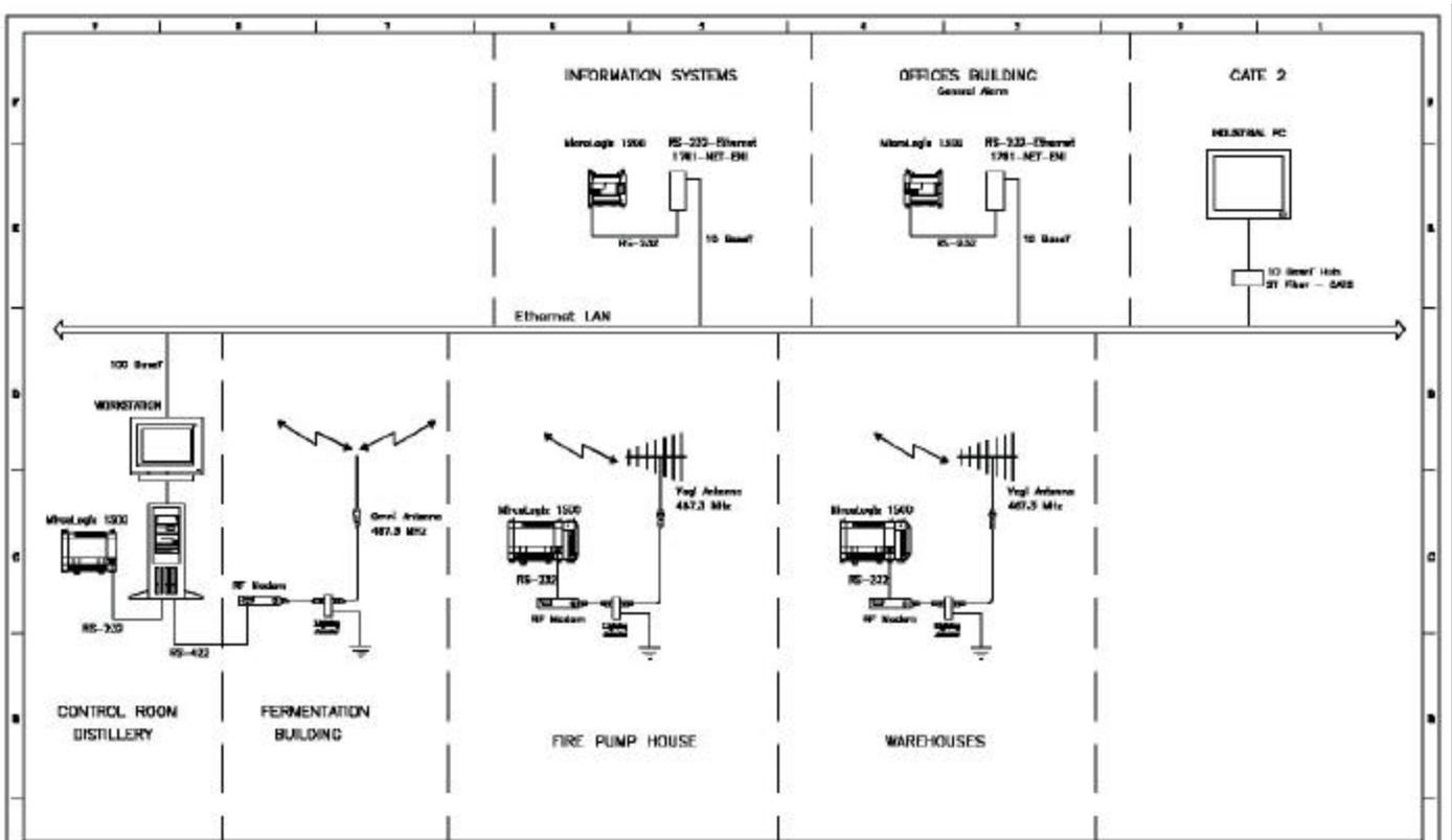
**Figure 3: Bacardi, Puerto Rico Site Diagram**
