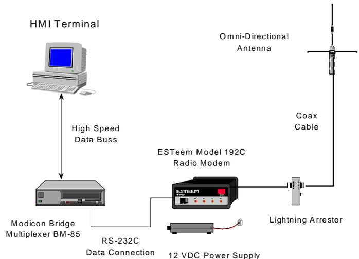
**Figure 2: Control Room Equipment Diagram**
