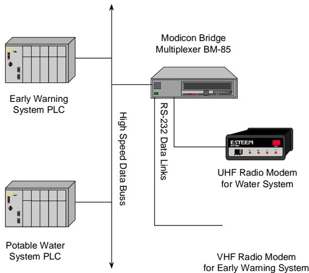
**Figure 3: Security Office PLC Network Diagram**
