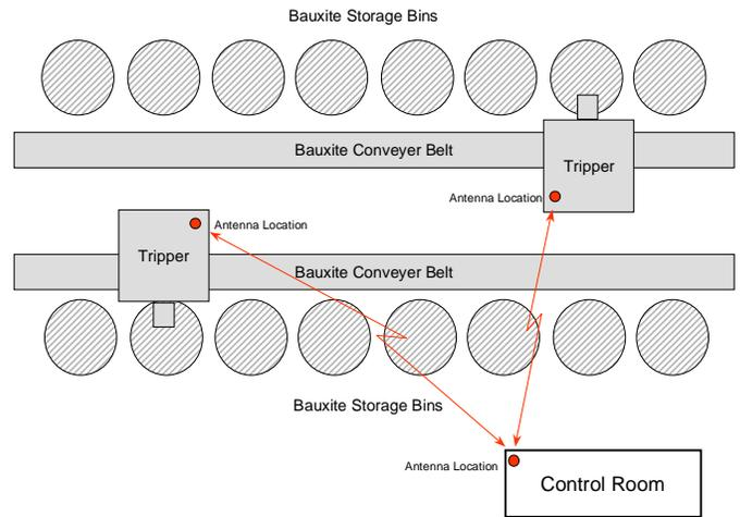
**Figure 1: Bauxite Reclaim System Diagram**
