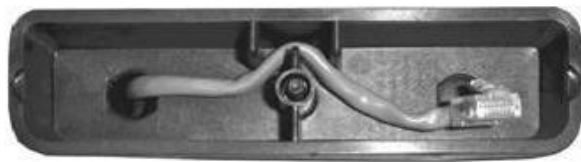
Route the cable through strain relief fins
