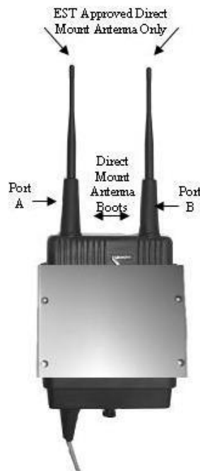
Figure 10: Antenna Connector Boot Installation
