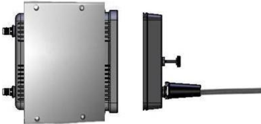
Figure 9: Face Plate Cover Installation
